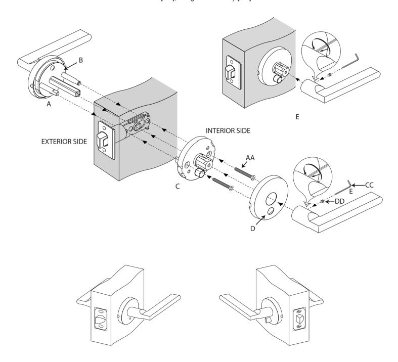
Note: To ensure correct alignment of the lever, tighten the mounting screws on the interior lock mechanism while holding the exterior lever upwards.
