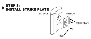
Secure the strike plate to the door jamb using screws [BB]
