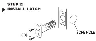
Secure the latch to the door edge using screws [BB] **Note:** The bevel (curved side) of the latch should be facing the door jamb when the door closes.
